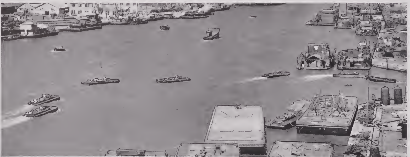
FIGURE 44. DUKWs operating in Manila Harbor, where damaged port installations made them necessary.
